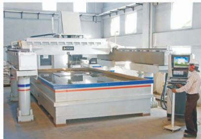
Water-jet cutting machine
