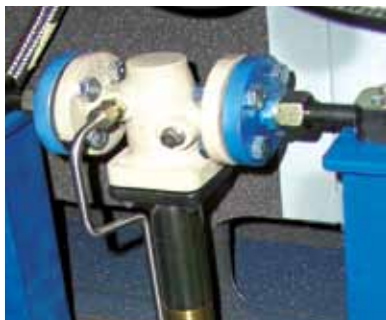
Sealing gas regulator for exhaust compression
