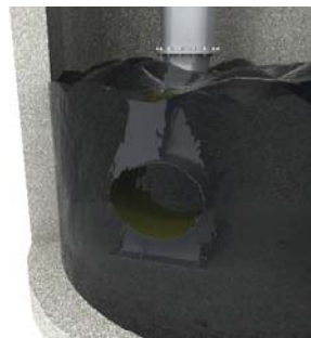
Energy Dissipation Unit during Air Entrainment Mode
